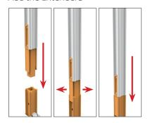
Slot the extenders into tripod, pulling clips apart until secured
